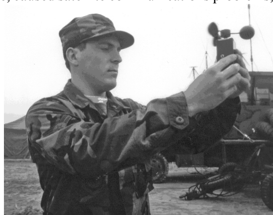
Figure 7-4: A1C Joey Mumm, 17th WS, Travis AFB, CA, measures wind speed using a Simms anemometer for a low altitude parachute extraction system drop, during TEAM SPIRIT 89 at Yoju extraction zone, KR. (MAC News svc) (USAF Photo by SSgt Mark Allen)
