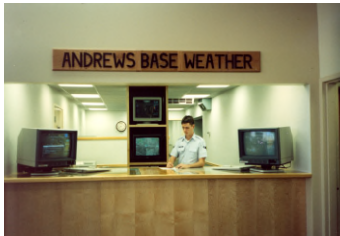
Figure 7-14: Andrews Base Weather Station briefing function AWDS displays – no more clipboards of teletype bulletins, maps displays, and teleautowriters.
