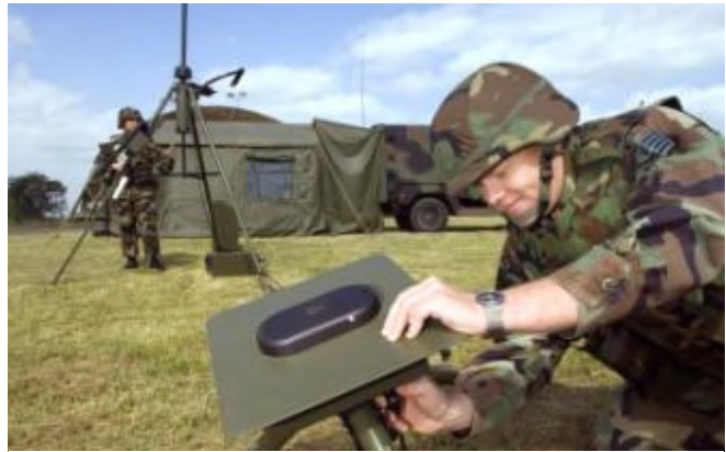
Figure 8-2: SSgt Craig Gaillardet attaches the lightning detector to the base unit of the AN/TMQ-53 Tactical Meteorological Observing System (TMOS). Sergeant Gaillardet, a combat weather forecaster with the 7th WS, and other members of his team conduct realistic training to optimize support to their supported US Army unit. (USAF photo by MSgt John E. Lasky)
