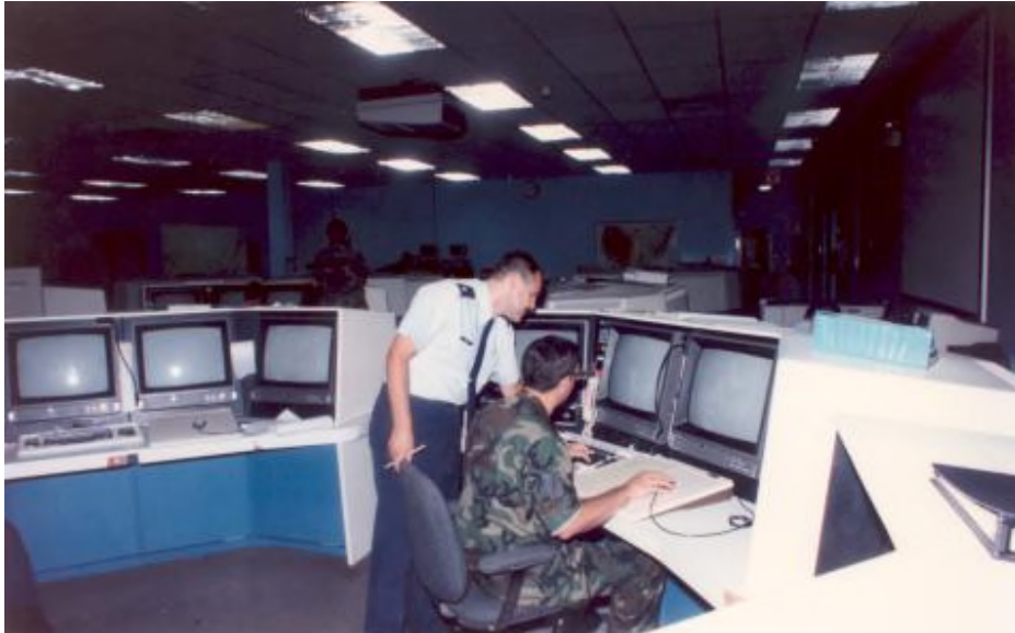
Figure 7-5: The revised “Floor” at AFGWC. SDHS Consoles arranged in groups redefined the look of the AFGWC “Floor” – gone were the large map tables, grease pencils, blue smocks, and acetate overlays.
