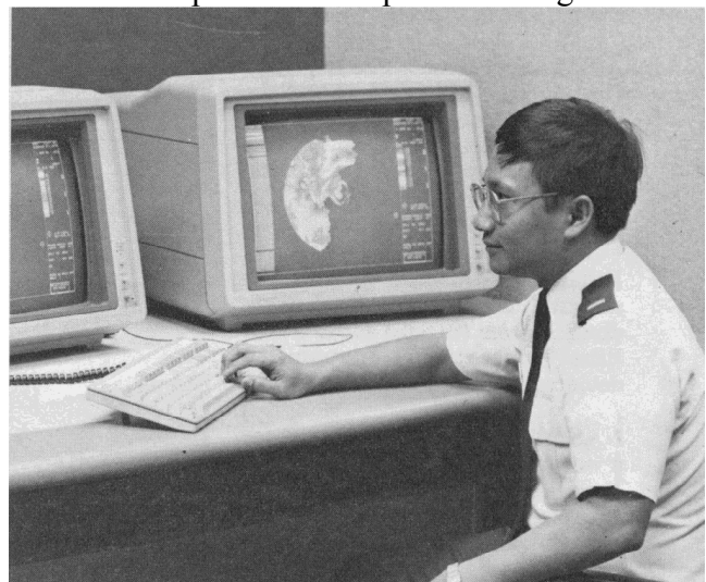
Figure 7-7: 2 nd Lt Nhung Nguyen, an AWS engineer assigned to AWS Ground Programs, Testing and Engineering Division, evaluates the NEXRAD Principal User Processor (PUP) subsystem.
