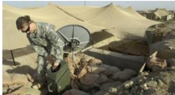
Figure 9-1: TSgt. Andrea Patterson, assigned to Forward Operating Base Kalsu south of Baghdad, Iraq, cleans debris from the lens cover on the cloud height detector of the AN/TMQ-53.
