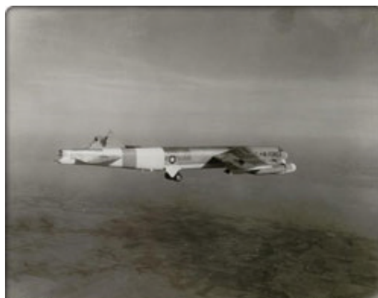
Figure 4-12: B-52H (61-0023), configured at the time as a test bed to investigate structural failures, still flying after its vertical stabilizer sheared off in severe turbulence on 10 January 1964. The aircraft landed safely.
