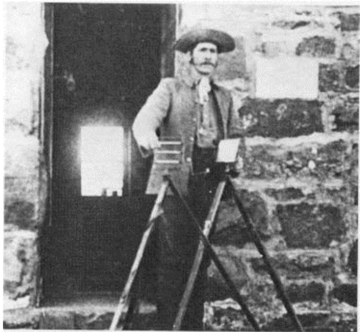
Figure 1-1: An U.S. Army Signal Corps soldier at Pikes Peak weather station, transmits latest weather data by heliograph (circa 1880s)
