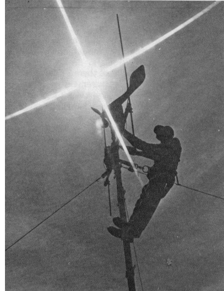
Figure 6-1: A weather equipment repairman aligns a T-755 Wind Sensor, a sub-system of the A/N-GMQ-20 Wind Set.
