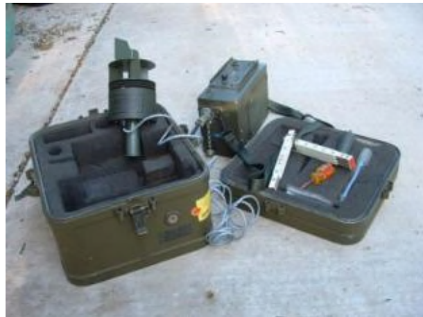
Figure 6-18: AN/TMQ-34, Meteorological Measuring Set. Carpenter's rule was used for snow depth measurement.
