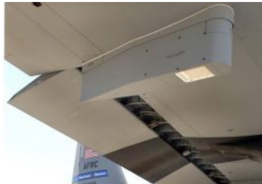
Figure 9-2: The Stepped-Frequency Microwave Radiometer installed under the starboard wing of a 53 rd WRS WC-130J. (Photo Courtesy of Lockheed Martin)
