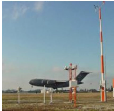
Figure-8-13: A C-17 Globemaster III touches down at McCord AFB, WA as the AN/FMQ-19 Automatic Meteorological Station creates an automated surface weather observation. Located near the touchdown point of the runway, primary sensors visible are, from left, precipitation, lightning detection, cloud height, combined visibility/present weather, and wind direction/speed [atop the 10 meter mast].
