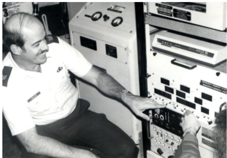
Figure 7-6: MSgt John Carlson explaining FMQ-13 wind system indicator to SSgt Katherine Zupan. Recorder [on top of indicator] was a dot matrix printer. (USAF Photo)
