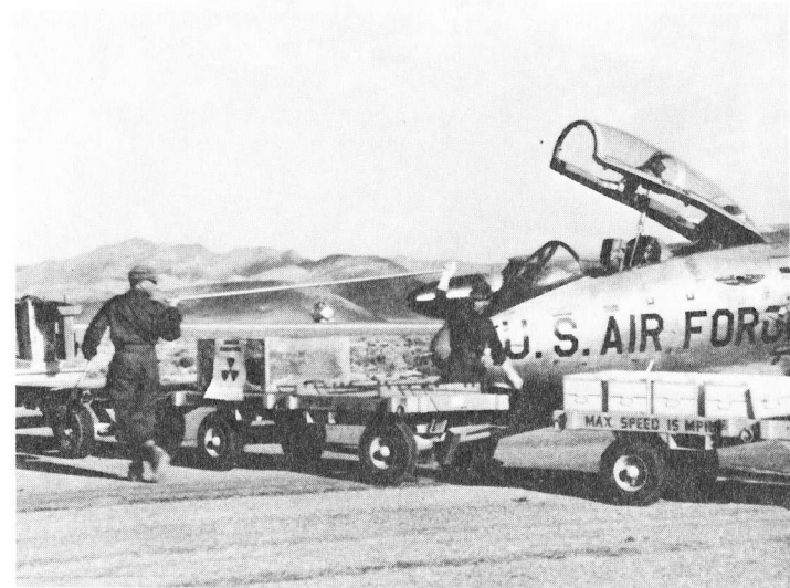
RADIOACTIVITY. Two airmen transporting a "pig", a lead container for hot samples, to shipping containers on the trailer at far right. The samples were taken from the B-57 shown in the background which just returned from penetration of an atomic cloud on March 28th, 1957, to gather samples for AEC studies, Operation Plumbbob.
