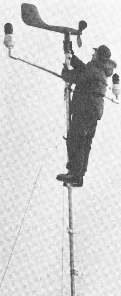
AN/GMQ-11 wind sensing equipment being checked for orientation by a weather maintenance man at Elmendorf AFB AK.
