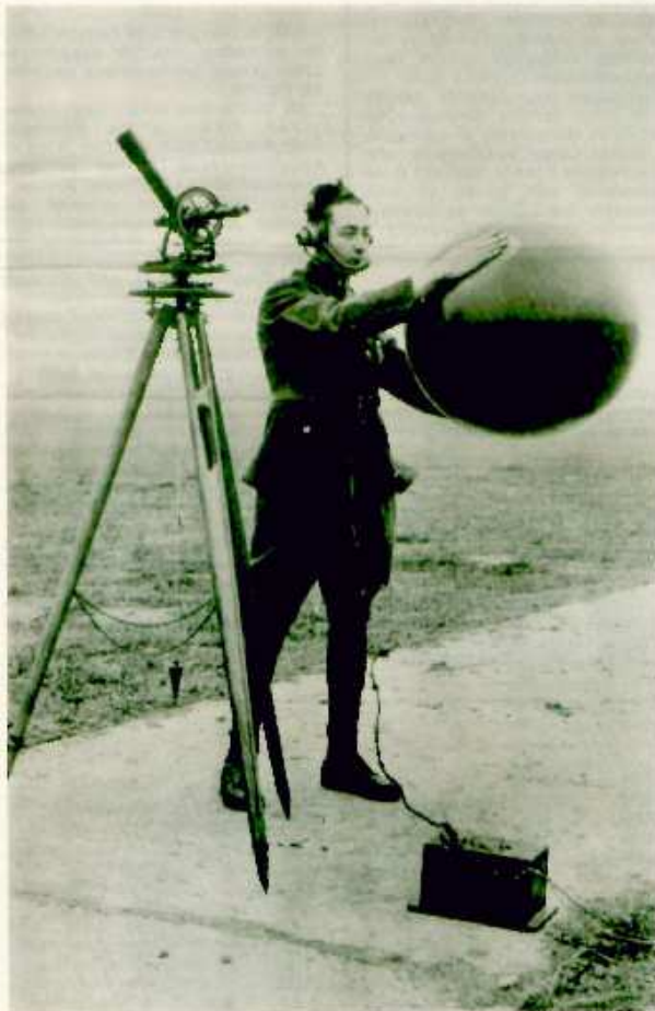
U.S. National Archives photo With theodolite and pilot balloon, a military weatherman of the era between World Wars I and II gets ready to launch a probe of the atmosphere above the surface. He will track the balloon's flight using the three-legged theodolite.
