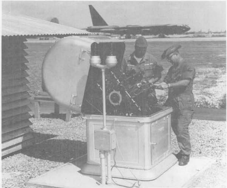
Adjusting AN/GMQ-13 rotating beam ceilometer at U-Tapao RTNAS, Thailand, in 1969 are Sgts Raymond J. Metzge (left) and Robert W. Stalker from Det 30 of 1WG's (1WW) 10WS. In background is SAC B-52 on landing roll.
