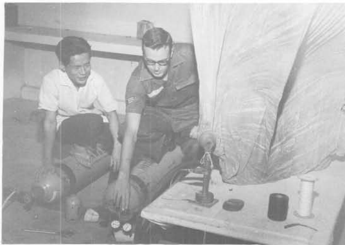
A1C Raymond J. Braun regulates flow of hydrogen into a weather balloon at Da Nang AB, RVN. Studying the operation is Ngo T. Phat, a civilian rawinsonde operator of the Vietnamese weather service.
