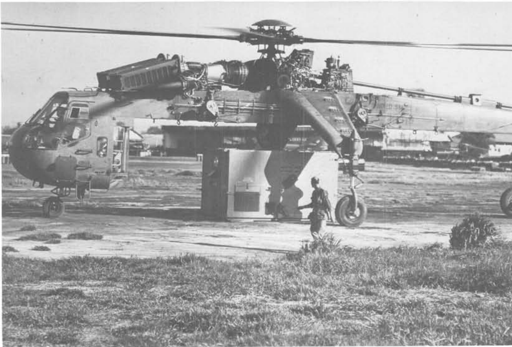
AN/MMQ-2 meteorological van being moved by an Army CH-54 "Flying Crane," from Tan Son Nhut to Long Giao.
