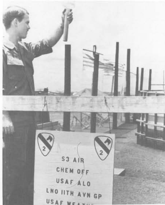
With the 1st Cavalry Division's 2d Brigade at Phuoc Vinh in September 1970, Sgt Ralph T. Wilson, a weather observer with the 5th Weather Squadron's Operating Location B, twirls a sling psychrometer, left, and examines his rain gauge, right. In the background are Viet Cong weapons captured by the brigade.
