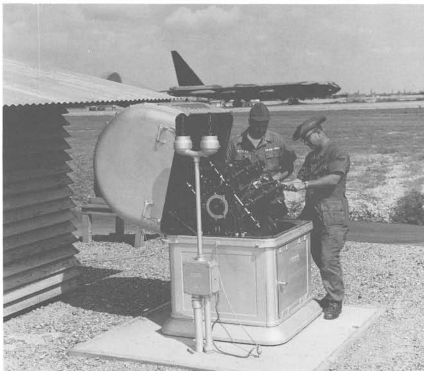
Above, adjusting AN/GMQ-13 rotating beam ceilometer at U-Tapao RTNAS, Thailand, in 1969, are Sgts Raymond J. Metzge (left) and Robert W. Stalker from Det 30 of the 10th Weather Squadron. In background is SACB-52 on landing roll. Below, wind information from Pibals launched at this site at U-Tapao helped in the preparation of ballistic winds forecasts for C-130 airdrops over neighboring Cambodia.
